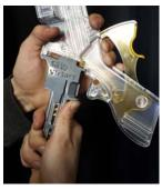
Be sure to have 10 shells lined up before loading and hold loader vertical.
