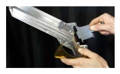
Insert your magazine through the small ring into the adapter until it latches into notch. The follower of your magazine will be pushed down when this is done
