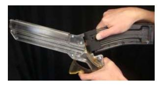
To remove the magazine, while holding like pictured above, gently press down on latch and pull out on the magazine.
